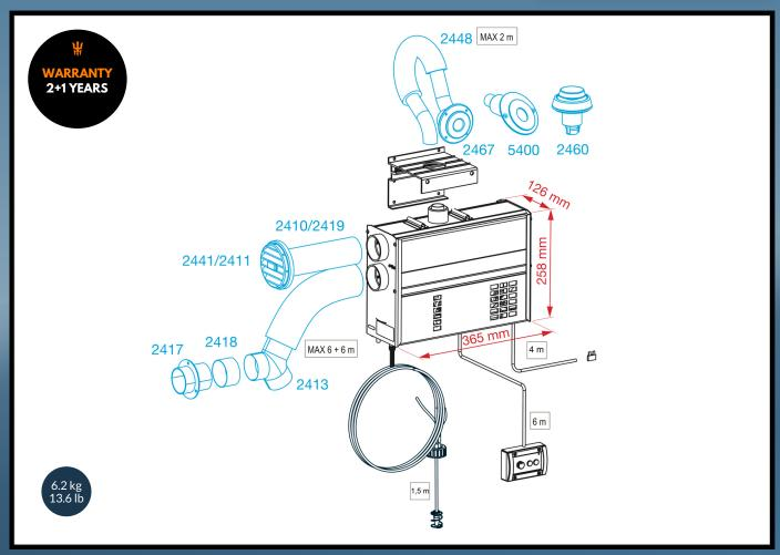
Accessories in black come with the standard package. Accessories in blue are additional. The calculated values are measured in a reference measurement wall, which is constructed to respond to a typical boat installation. The technical values have been measured with the maximum length of ducting, exhaust pipe, fuel line, and power cord. The figures allow for 10 % reserve - yours may vary.
